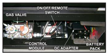
Figure 11.1. Valve Components
